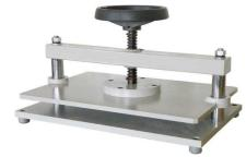
It is made in stainless steel, height and pressure can be adjusted by hand wheel. Most pressure can reach up to two ton. Flatten area: 460×350mm Flatten height: 70mm Machine weight: 52kg Dimension: 530×350×300mm
