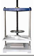
It is made in stainless steel, height and pressure can be adjusted by hand wheel. Most pressure can reach up to two ton. Flatten area: 500×450mm Flatten height: 500mm Weight: 110kg Dimension: 610×450×950mm
